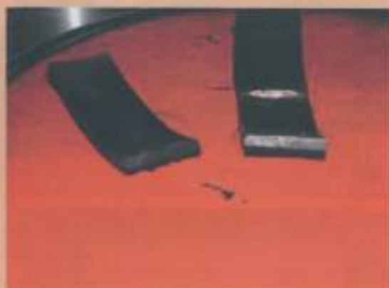
Bamboo Carbonization 320°C 20 minutes
